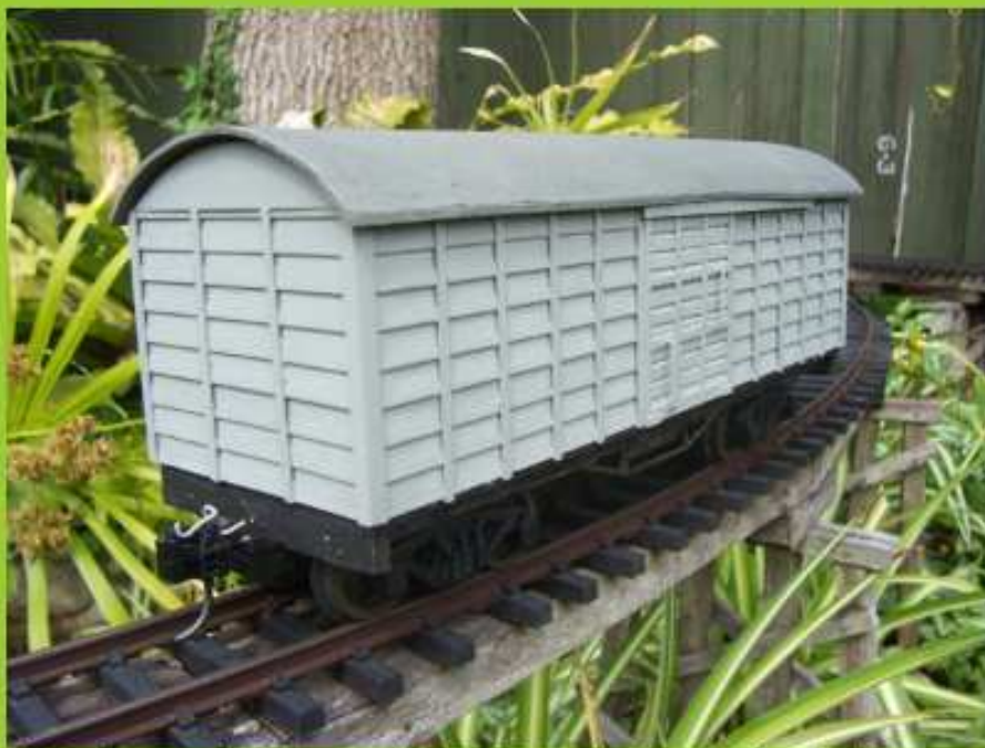
Made from wood and styrene, this is a foreshortened model of a QR CLC wagon.
