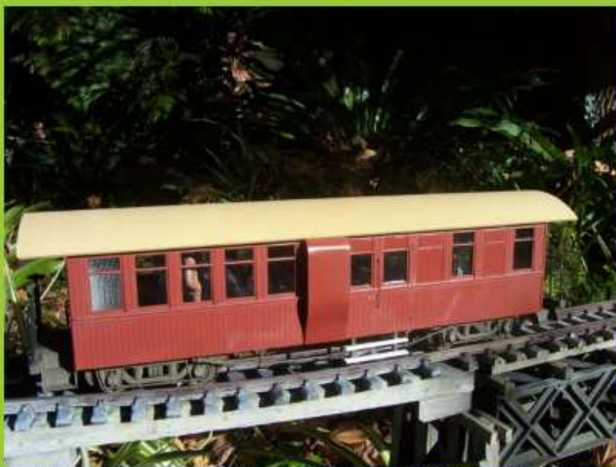
A Bachmann coach has been modified to resemble a CLV / BLV Guards Van. This will allow use in mixed train traffic to cater for more passengers.
